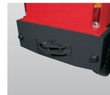
Easy-disconnect trailer coupler (NTF200P)
