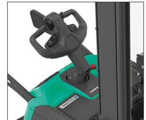
Power steering tiller arm
